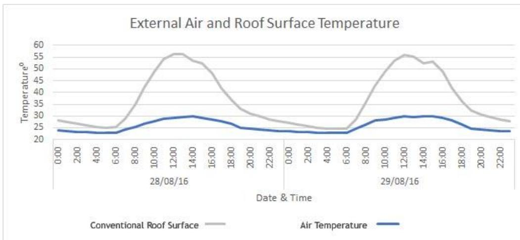
Figure 15 External Air and Conventional Roof Surface Temperatures
