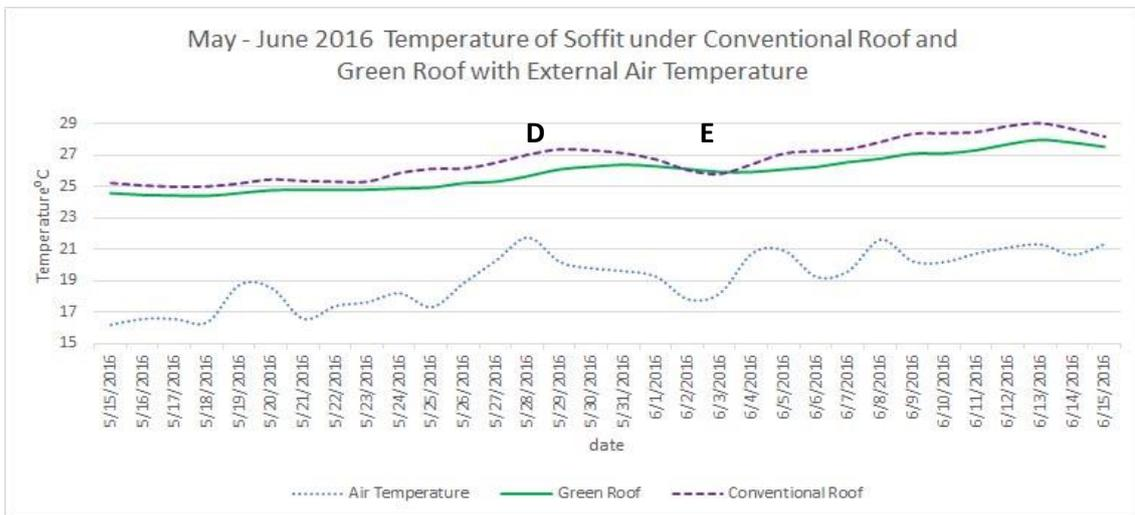
At the end of the test period in August the ambient air temperature reached the highest external air temperature of 34.43°C at 13:00hrs. on the 1<sup>st</sup>. of August. Again the green roof temperatures appear more stable.
