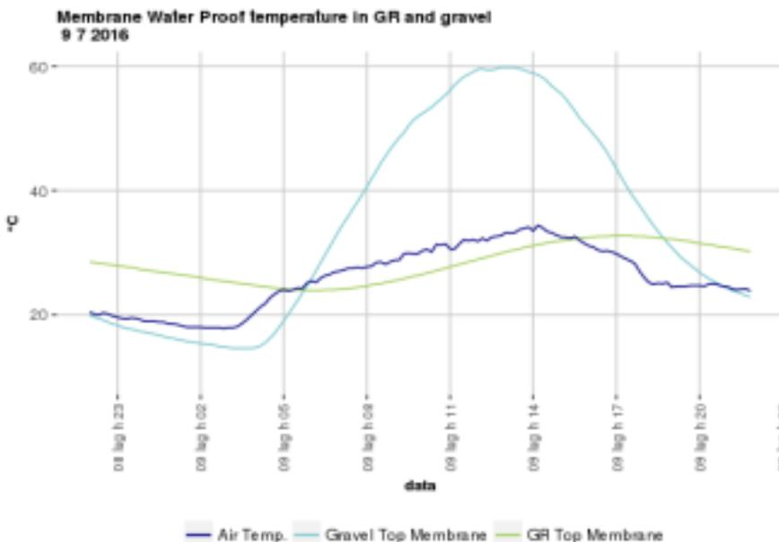
Figure 45 One day sample of Membrane temperatures in summer
