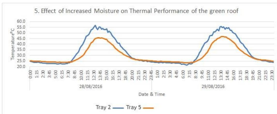
Figure 20 Graph showing the effect of moisture on the absorption of heat at the surface of the planting medium
