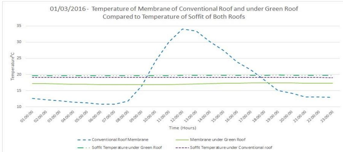
Table 23 Comparing temperatures of the membrane and soffit beneath the green roof and conventional roof.
