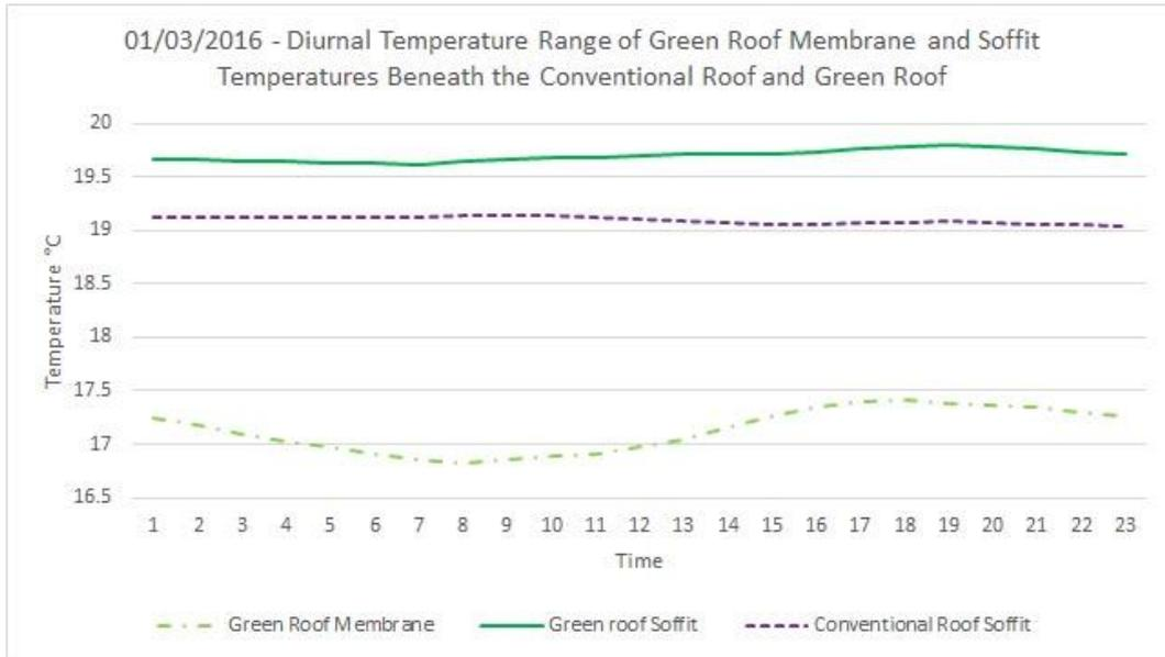
Figure 38 Graph of the diurnal temperature range of the green roof membrane and soffit temperatures beneath the conventional roof and green roof.
