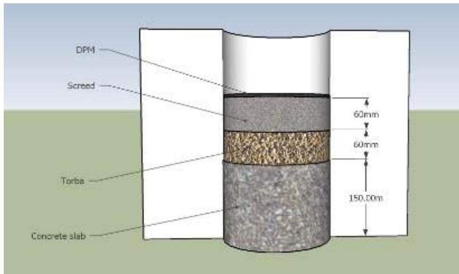
Figure 55 Traditional slab roof / 'U' value = 2.3
