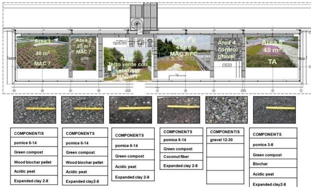
Figure 41 Plot layout of the Minoprio Green Roof, Area 2 is the GR monitored area, Area 4 is the reference area covered with gravel.
