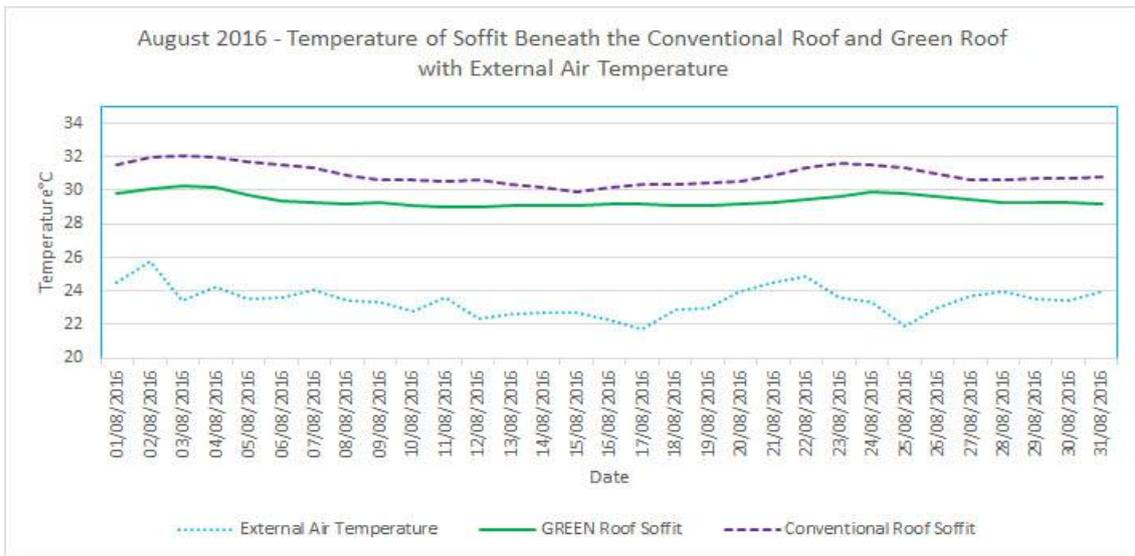
Table 20 below illustrates the range of temperatures measured under the soffit of the green roof compared to that of the conventional roof.
