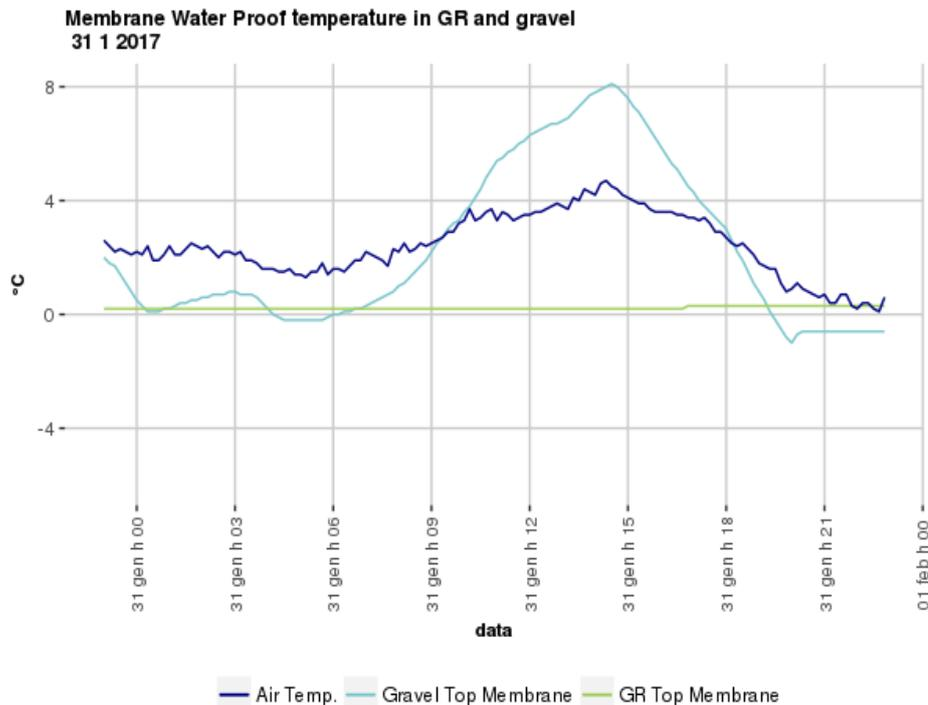
Figure 47 One day sample of Membrane temperatures in winter
