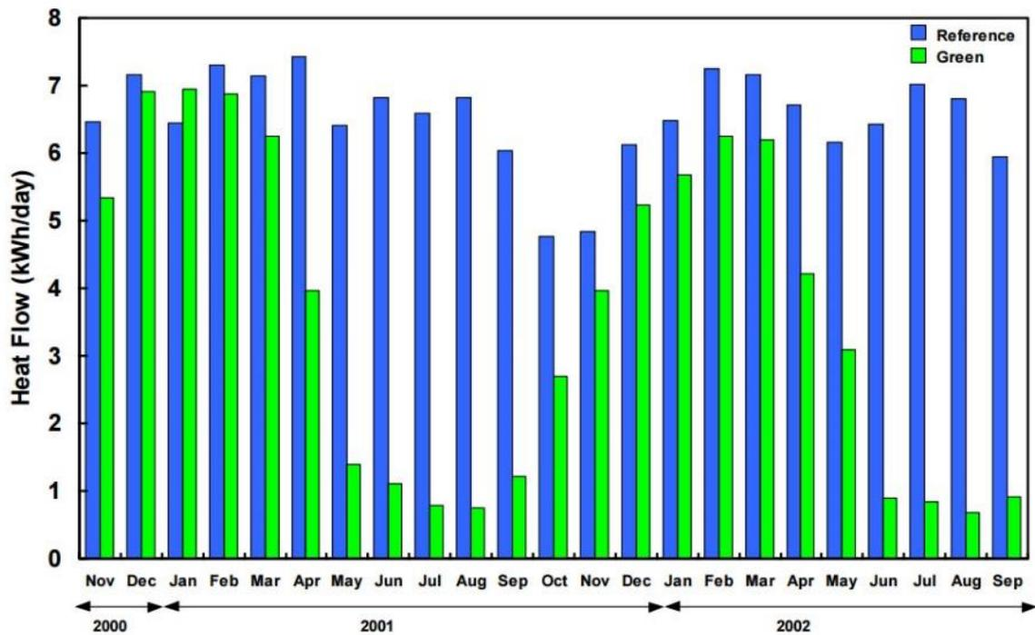
Figure 4 Heat flow measurements showing that the average daily energy demand due to the heat flow through the Green Roof was significantly less than that of the Reference Roof in the spring and summer. (Liu, 2003)
