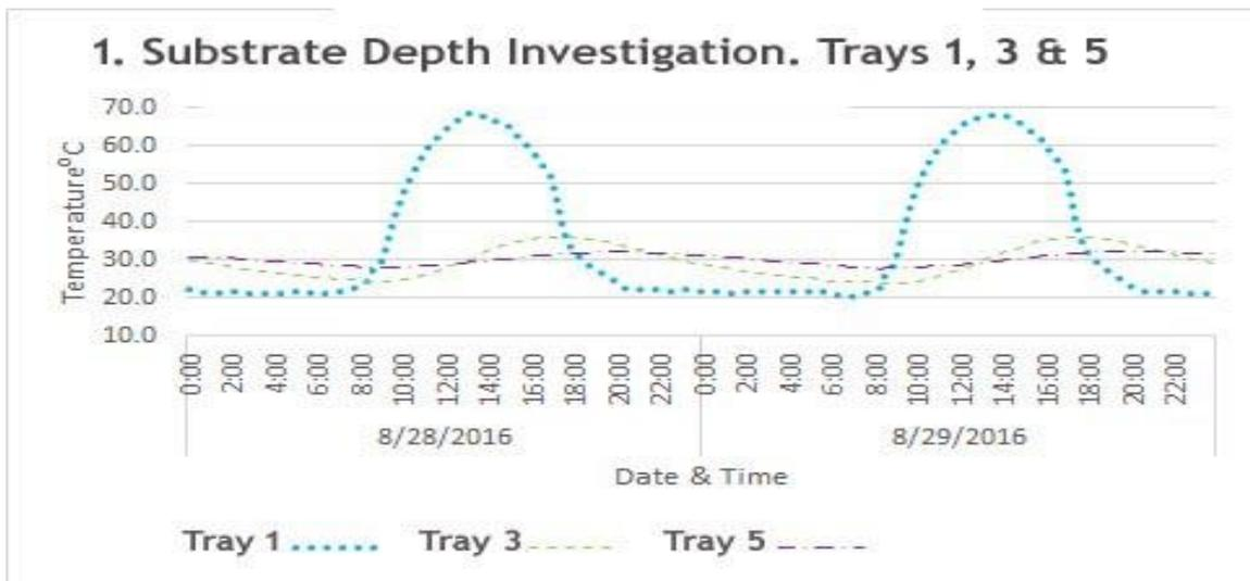
Figure 14 Investigation 1 - Comparison of solar gains in Trays 1, 3 & 5 of varying substrate depths over two days 28/08/16 and 02/09/16.
