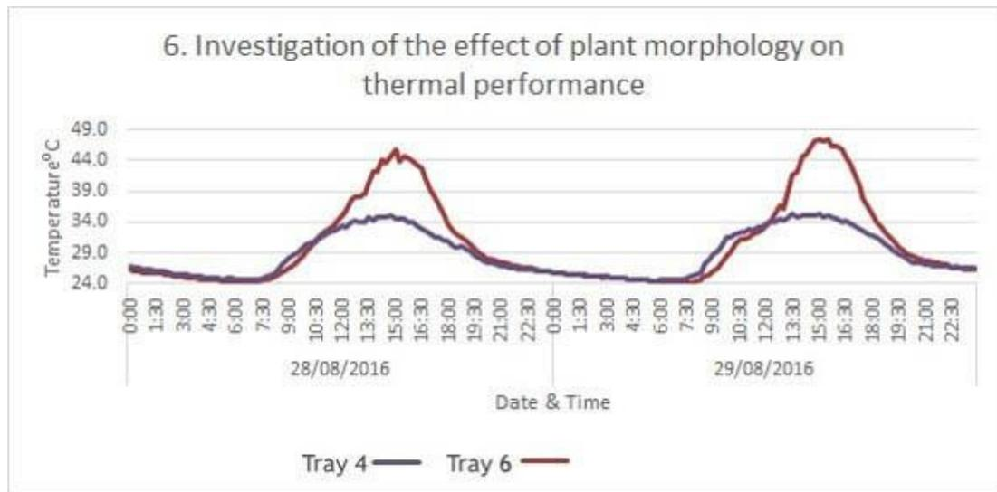
As with investigation 4, the Sedum sediform provided better insulation from solar heat gains at the surface of the growing media. It is thought that this is due to the more intense coverage of the growing media surface by this particular plant when compared to Phlomis fruticosa.
