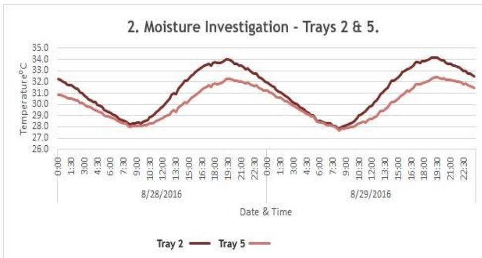
Figure 16 Investigation 2 - Graph comparing Thermal performance of Trays 2 (Dry) and 5 (Irrigated).
