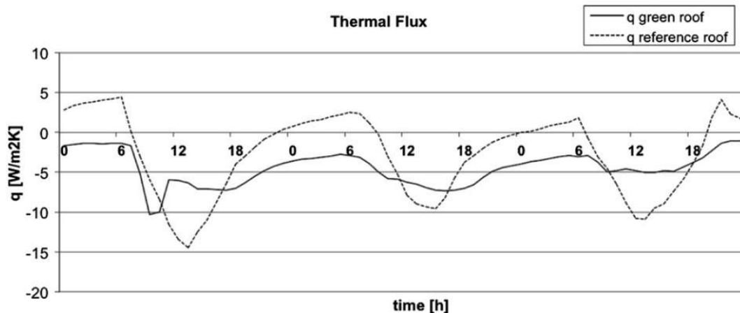
Figure 8 Heat flux measured on the internal surface of the green roof and the reference roof at the Regional Council of Marche (Italy). (R. Fioretti, 2010)
