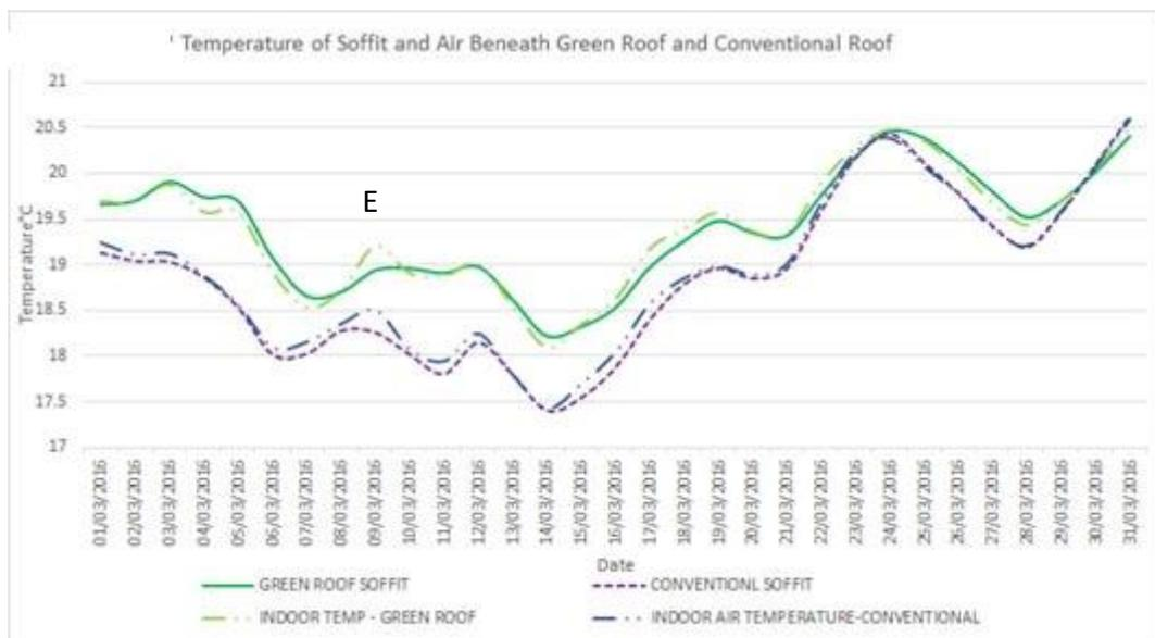
Figure 39 Temperature of Soffit and ambient air beneath green roof and conventional roof
