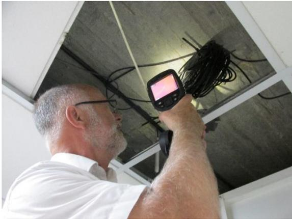
It was decided to take thermal camera images of the soffit under the conventional roof and the green roof in order to get an initial indication of the likely temperature ranges that could be expected. A FLIR E60 thermal camera was used to capture the images at noon on the 12th of May 2106.
