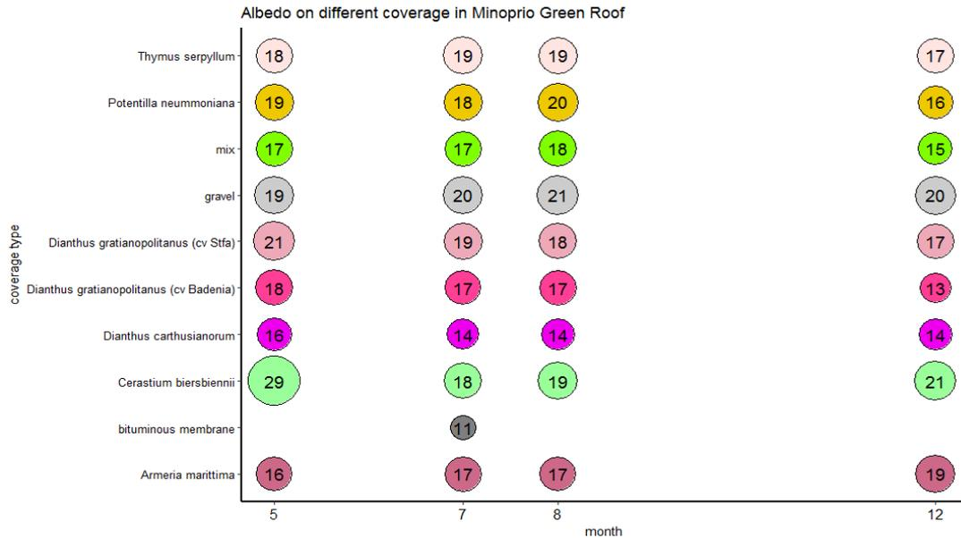
Figure 43 Albedo recorded on various surfaces on the roof at Fondazione Minoprio.
