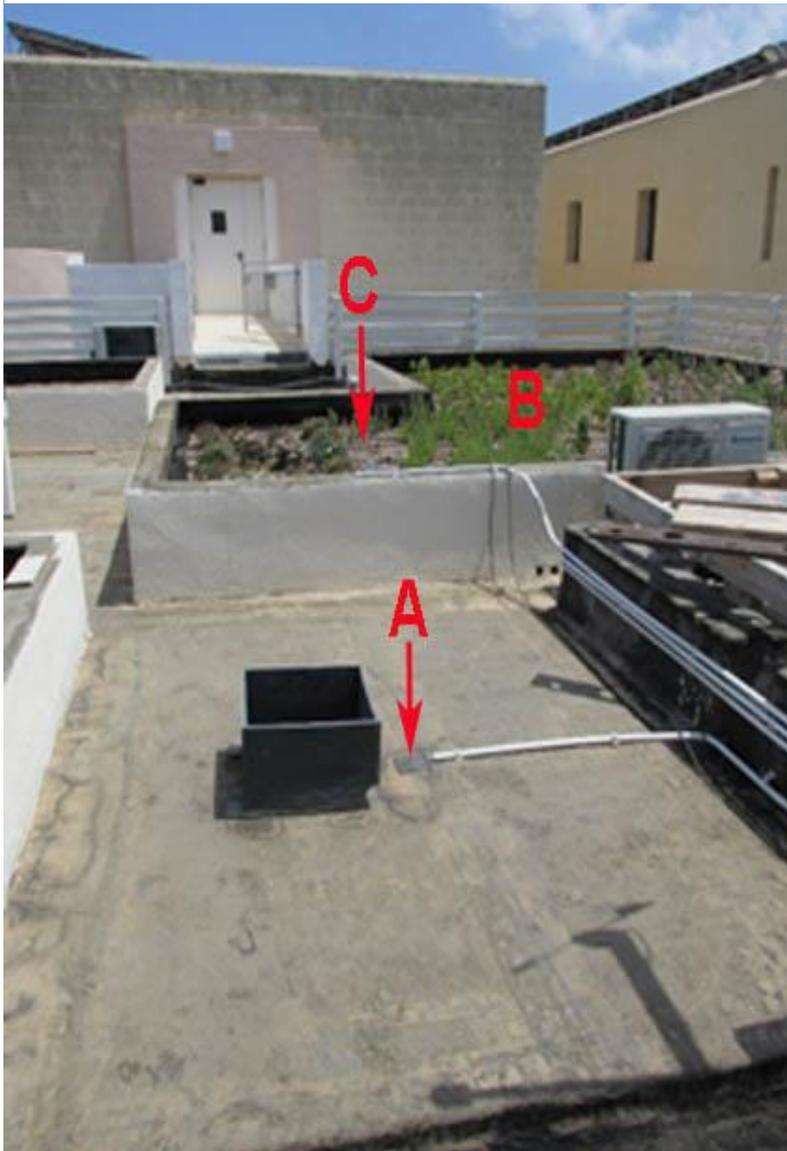
A = Thermocouple attached to the external surface of the conventional roof. An additional thermocouple and heat flux sensor were attached to the ceiling directly under this position (see Fig. 24).
